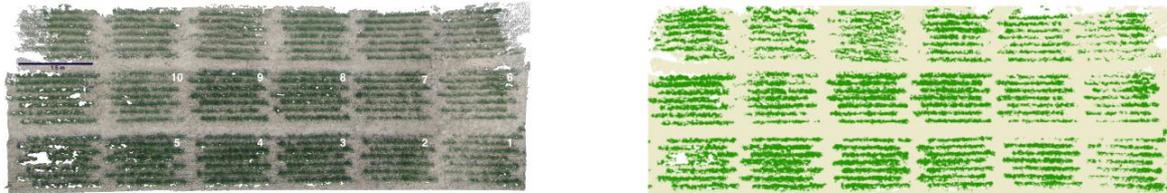
**Figure 3:** Left: Dense point cloud of a winter wheat genotype trial generated from aerial images using Pix4Dmapper by Pix4D. The numbers indicate the plot indices used for referencing. Right: Segmented point cloud generated using automated thresholding based on the excess green index and Otsu's method. Green points represent winter wheat and pale brown represents background.
