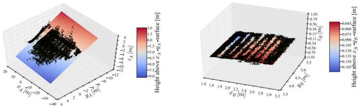
**Figure 5:** Left: Linear approximation of the ground surface to determine a scene's global orientation. One can observe the large variation in  $z$  coordinates creating the need for local regression surfaces for accurate height estimation. Right: Local regression surface along with the corresponding ground points from the point cloud for one plot. From KHANNA *et al.* 2015.
